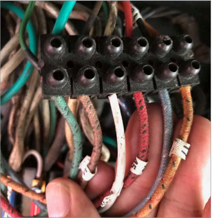
With the red wire removed, the wipers stopped – putting an end to what ended up being a bad ground.
